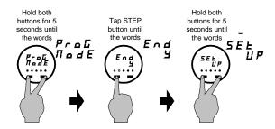
Setting Tank SIZE for the first time. Hold the STEP button in and power up to see and set size or use procedure below.
